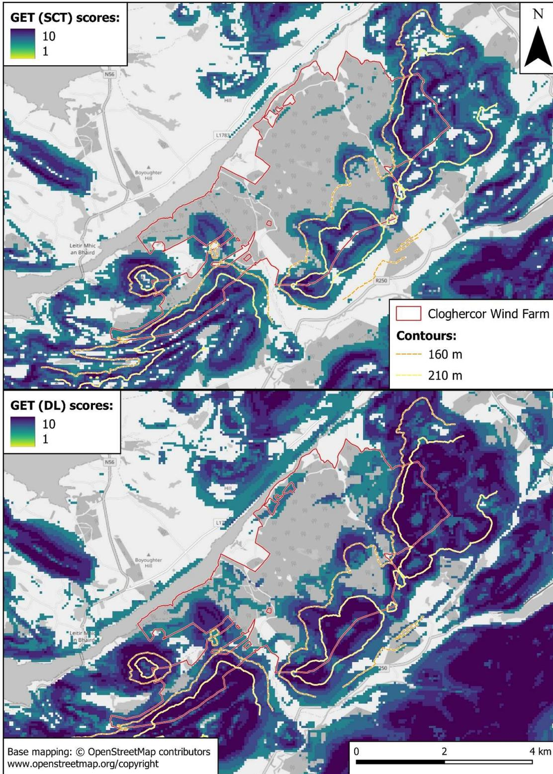
Figure A7.6.3 - Golden Eagle Topography (GET) modelling of the Cloghercor Wind Farm site, showing only scores  $\geq 6$ .
